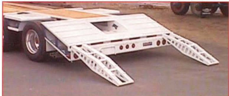
Low loading angle with ramps in place 15.25°
