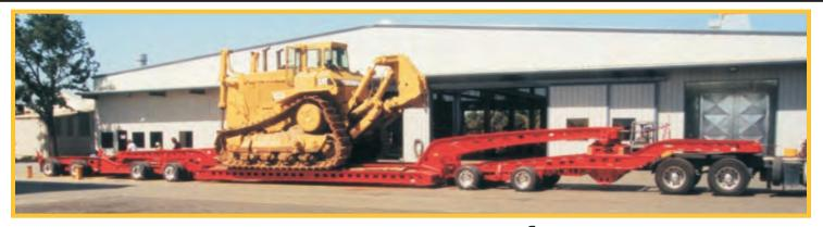
**88-Ton Payload** (in CA, with 16-tire jeep and 27ft deck) **Carry** D-10's and 375 Excavators!
