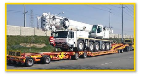
This 20" Hydraulic Lift with ratchet like lock support requires No Blocking. The low profile Rear End allows easier transporting of longer loads.
