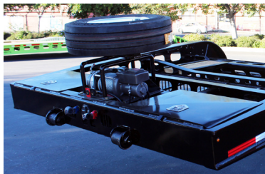
Electric Winch, Spare Tire w/ Mount , & Lockable Tool Boxes
